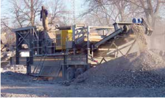
Figure 9 Crushed concrete from other sources can serve as recycled aggregate. (Courtesy Portland Cement Association)
